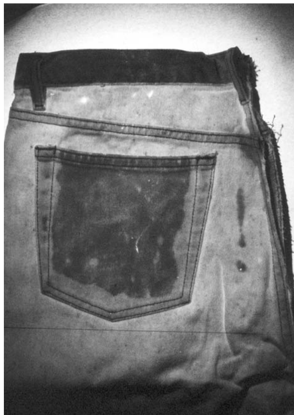
FIG. 1—Photograph of jeans impregnated with cocaine; darker areas corresponding to where cocaine was absent.
